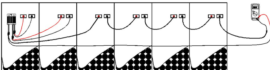
Figure 7.5-1 Optimizer string voltage test chart
