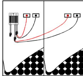
Figure 3.1-1 Schematic diagram of the optimizer and component wiring
