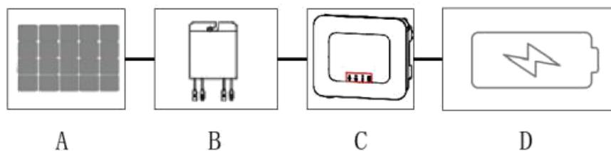
Figure 2.1-2 Application scenarios of optimizers in off-grid PV systems
