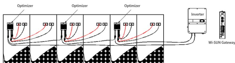
Figure 2.3-1 Wiring diagram of scheme 1
