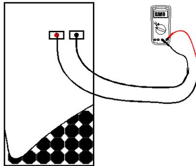
Figure 7.1-1 Schematic diagram of testing the voltage of photovoltaic modules
