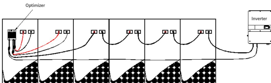
Figure 2.3-4 Wiring diagram of scheme 4
