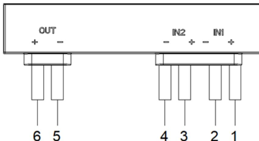
Figure 2.2-1 Schematic diagram of the optimizer interface
