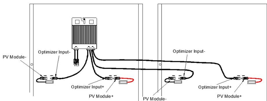
Figure 7.2-1 Schematic diagram of the optimizer connected to a PV module
