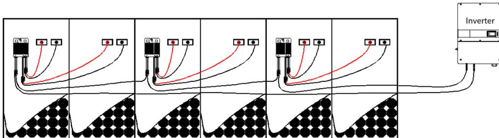
Figure 7.6-1 Schematic diagram of string access to inverter
