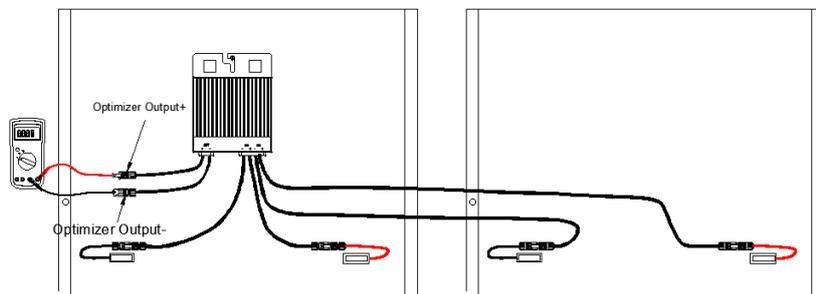
Figure 7.3-1 Schematic diagram of the output voltage test of the optimizer
