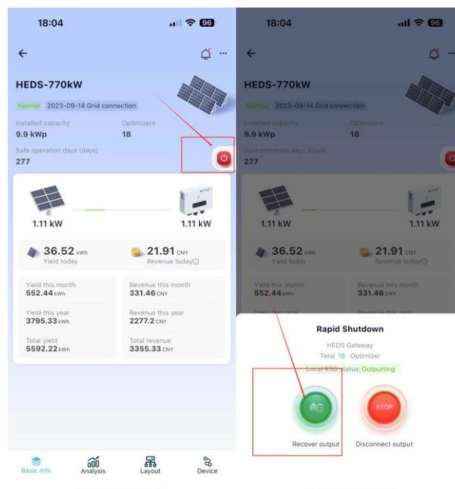
Figure 9.2-1 Output diagram of APP operation recovery
