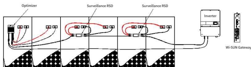
Figure 2.3-2 Wiring diagram of scheme 2
