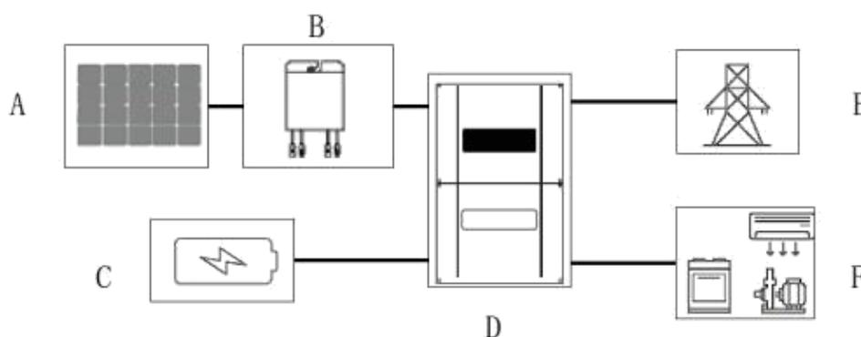
Figure 2.1-3 Application scenarios of optimizers in optical storage systems
