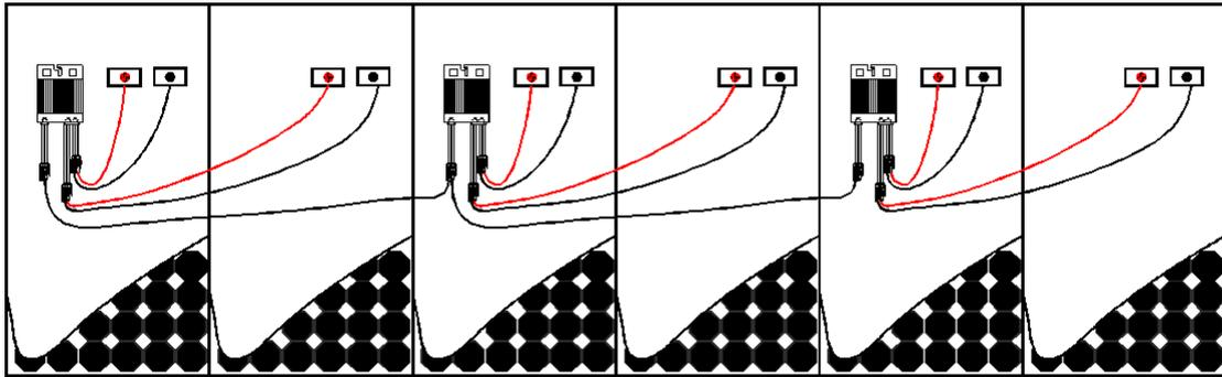
Figure 7.4-1 Schematic diagram of the optimizer connection
