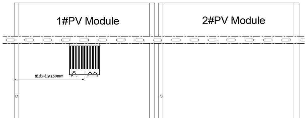
Figure 6.1-1 Schematic diagram of the installation location
