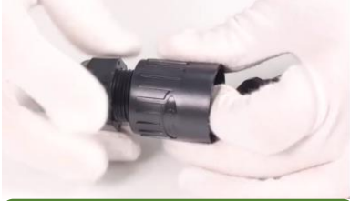
Unscrew the RJ45 plug bottom cover
