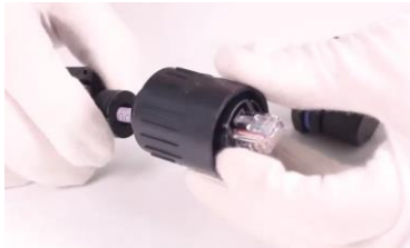
The network cable passes through the connector
